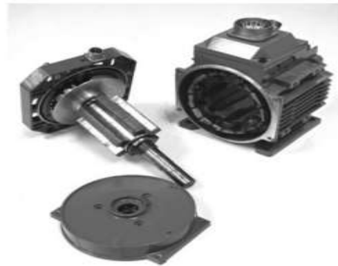
Fig. 1 Photograph of the 8/6 SRM disassembled
